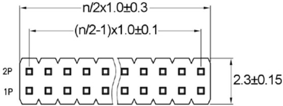
Recommended P.C.B Layout(Top Side) (PCB BOARD TOLERANCE±0.05)
